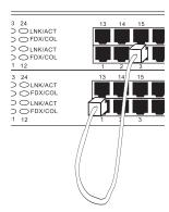
Each port supports Auto MDI & MDI-X functionality. When cascading with other switches or hubs, each port can connect directly to a switch or hub with straight through twisted pair cable.
